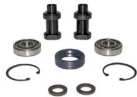
**109671ALT Cab Suspension Repair Kit**
